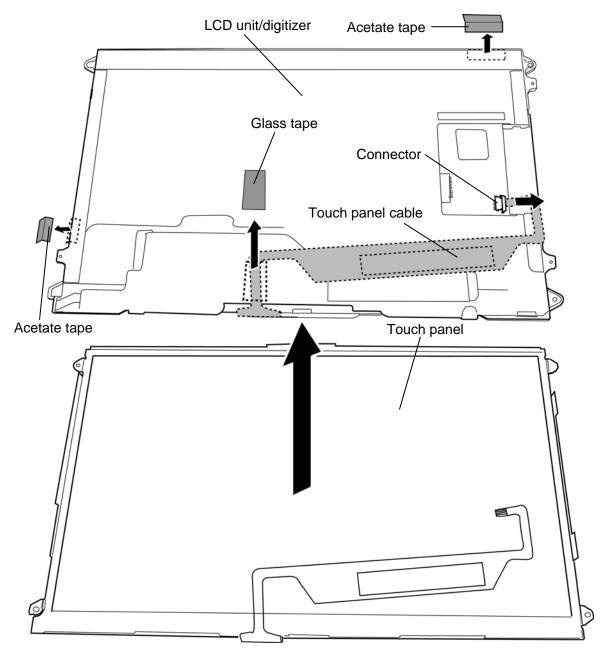
Figure 4-54 Removing the touch panel
